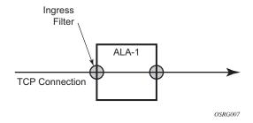
Figure 27: Applying an IP Filter to an Ingress Interface
